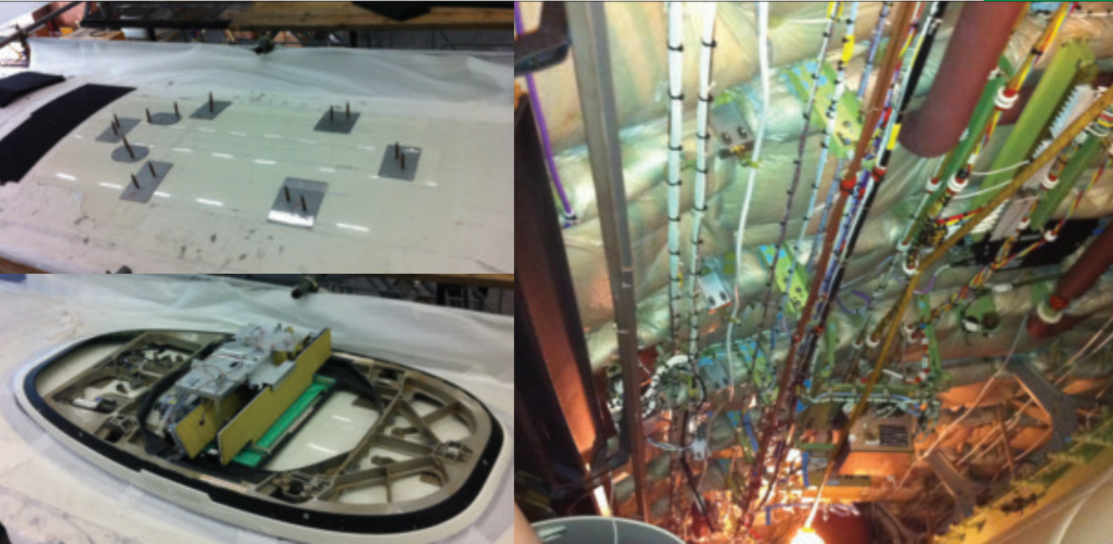
From left: Engineers from Turkish Technic were involved throughout the STC process; Centre: After the installation of external fittings and doublers, the adapter plate and the adapter plate skirt installed. After the application of required preventive compounds the antenna installed on the adapter plate. Right: Leaky feeder cables and data cables were installed for the GSM system through the cabin.
